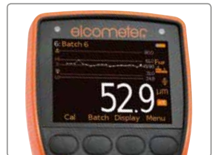
On-screen trend graph displaying last 20 measurement values
